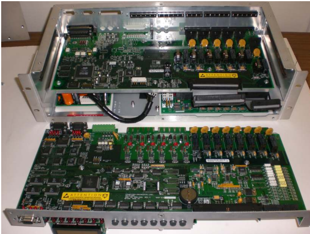
Figure 5-4. Inside the SEL-311L electronic relay unit.
